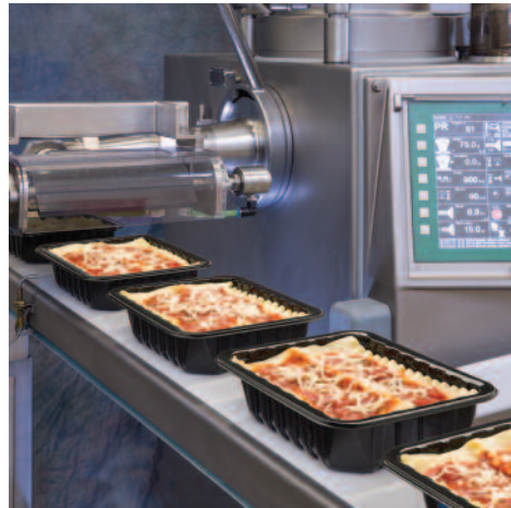
Cheese Shredder Topper Extrude and deposit a precise portion of cheese shreds directly onto conveyed product with complete coverage and no mess.
