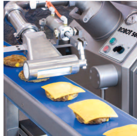
Cheese Slice Depositor Accurately form and deposit precisely portioned cheese slices onto conveyed product such as burgers and breads.
