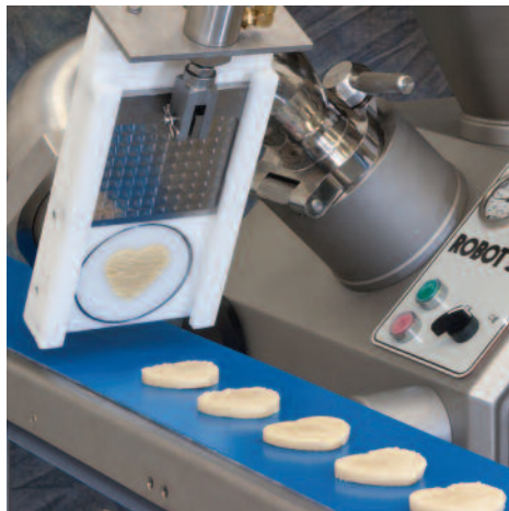
Cheese Shape Former Produce exact-weight formed cheese portions in all shapes and sizes – from unique shapes to sticks and planks.
