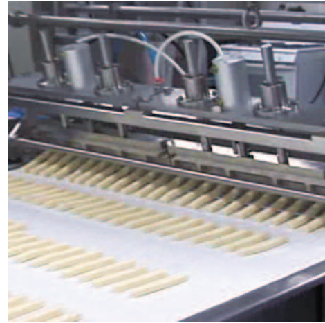
Multi-Outlet Cheese Extruder Multi-outlet waterwheel for high-volume production divides product flow into multiple lanes with equal portions from each outlet.
