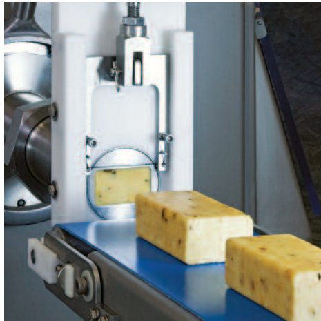
Cheese Block Forming Extrude exact-weight cheese blocks with consistent dimensions and clean, even ends from cheese offcuts and trim.
