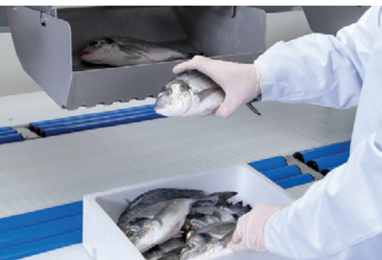
Optional tables & take away conveyor for finished products
