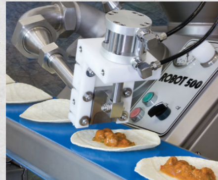
The Cut-Off Attachment produces portions of precise weight and size.
