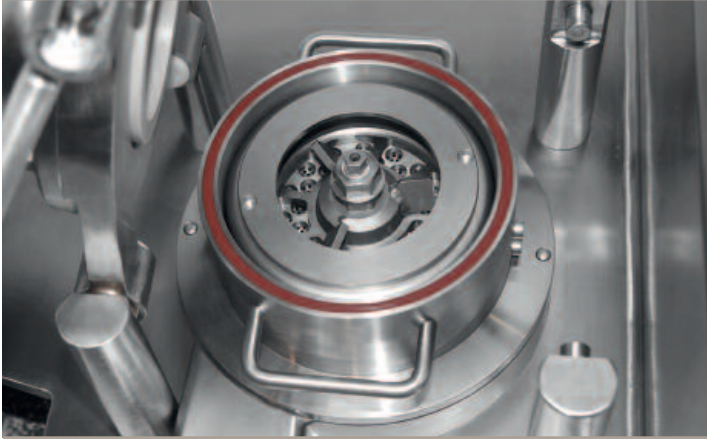
No metal-to-metal cutting plate contact
