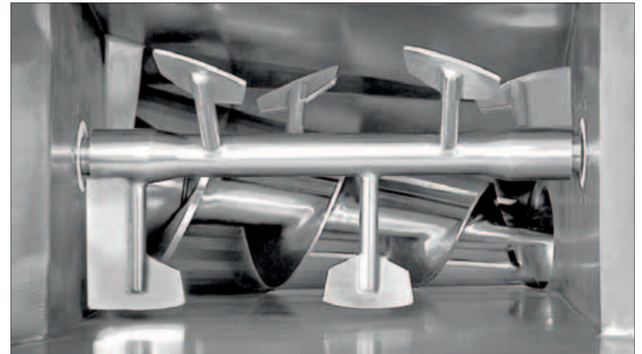
Automatic Mixing Grinder with mixing paddles
