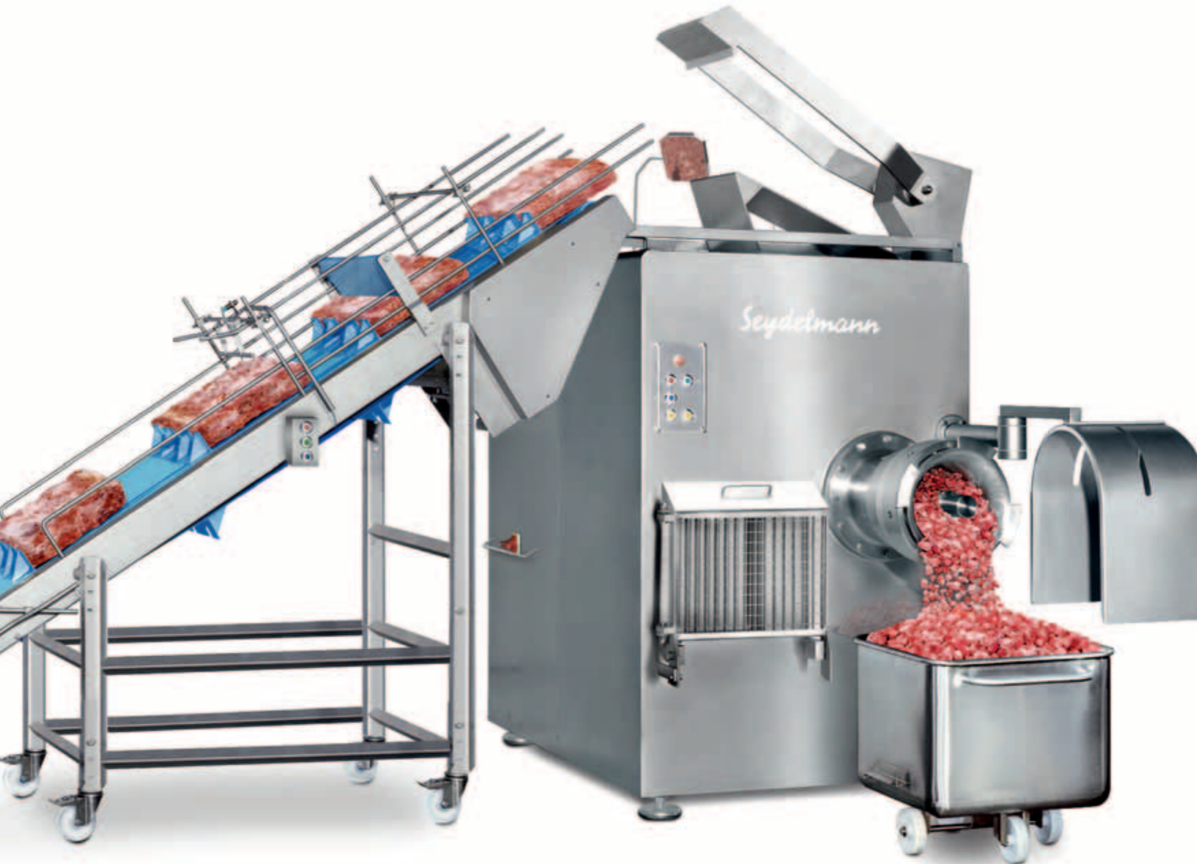
Frozen Meat Grinder GW 300 with angled conveyor belt.
