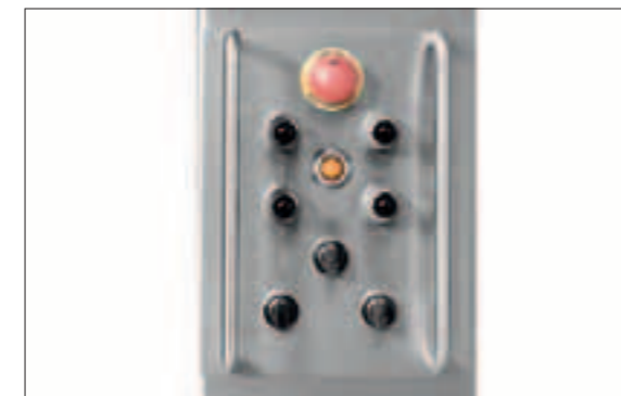
With frequency control motors the control panel also has cross switches.
