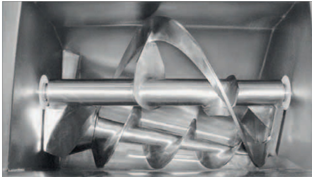
Automatic Mixing Grinder with mixing ribbon
